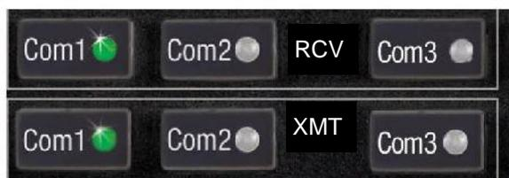
NOTE: Selecting COM 3 –TEL– mode will disable pilot and copilot intercom, as the intercom circuit is transferred to the telephone use.
