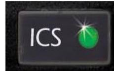
The front panel ICS switch controls muting of entertainment source #1 (for pilot and copilot). Pushing this button places the ICS in Karaoke (or sing along) mode, which inhibits the soft mute feature.
