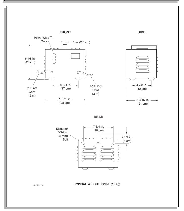
Fig. 38 PowerWise™ Portable Battery Charger Dimensions
