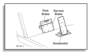
Fig. 6 Accelerator and Brake Controls
