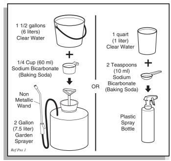
Fig. 27 Preparing Acid Neutralizing Solution
