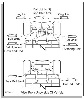
Fig. 20 Lubrication Points - Early Production
