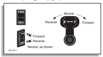
Fig. 5 Direction Selector Types
