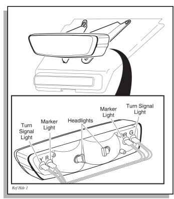
Fig. 12 Headlight, Turn Signal & Marker Light Bulb Replacement
