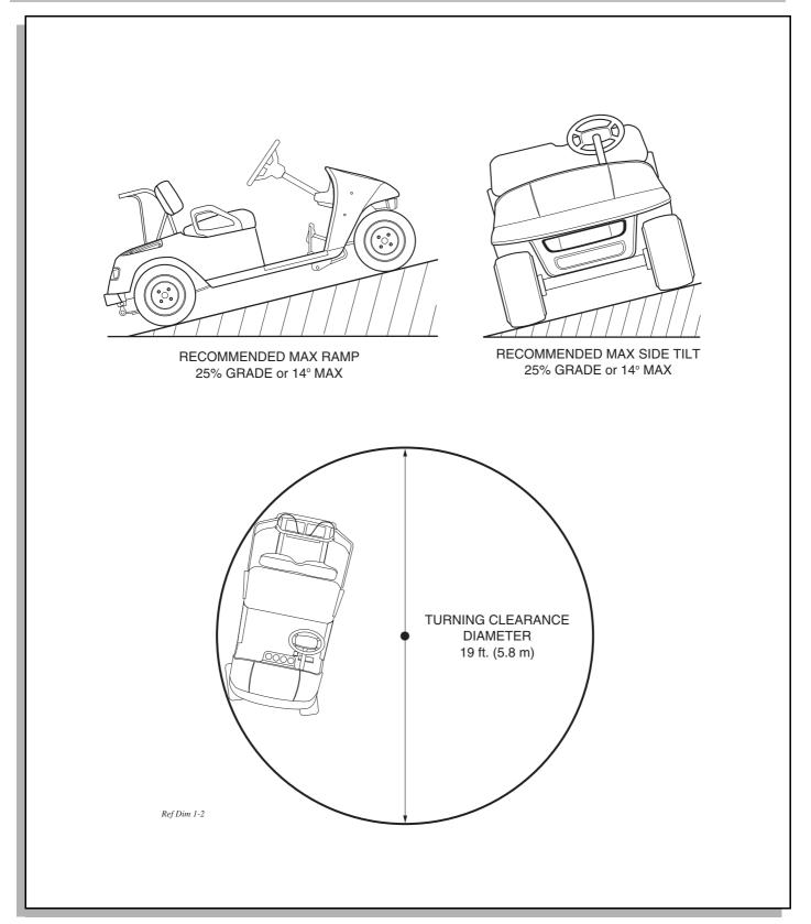
Fig. 37 Vehicle Dimensions, Incline Specifications and Turning Clearance Diameter
