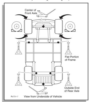
Fig. 10 Lifting the Vehicle
