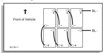
Fig. 28 Battery Connections
