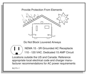
Fig. 2 Proper Charger Installation
