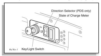
Fig. 4 Key/Light Switch & State of Charge Meter
