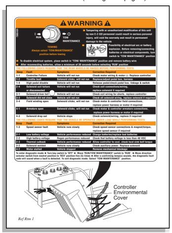
Fig. 7 Run-Tow/Maintenance Switch
