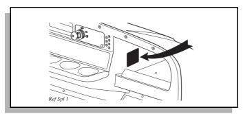
Fig. 14 Serial Number Plate Location - Early Production
