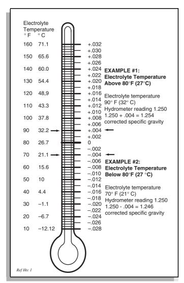
Fig. 31 Hydrometer Temperature Correction
