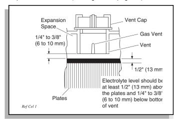
Fig. 24 Correct Electrolyte Level
