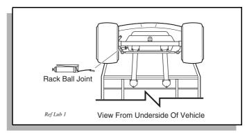
Fig. 21 Lubrication Points - Late Production
