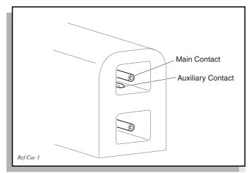
Fig. 32 Cleaning Auxiliary Contact in Charger Plug
