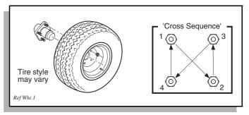
Fig. 11 Wheel Installation
