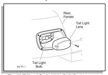
Fig. 13 Tail and Brake Light Bulb Replacement
