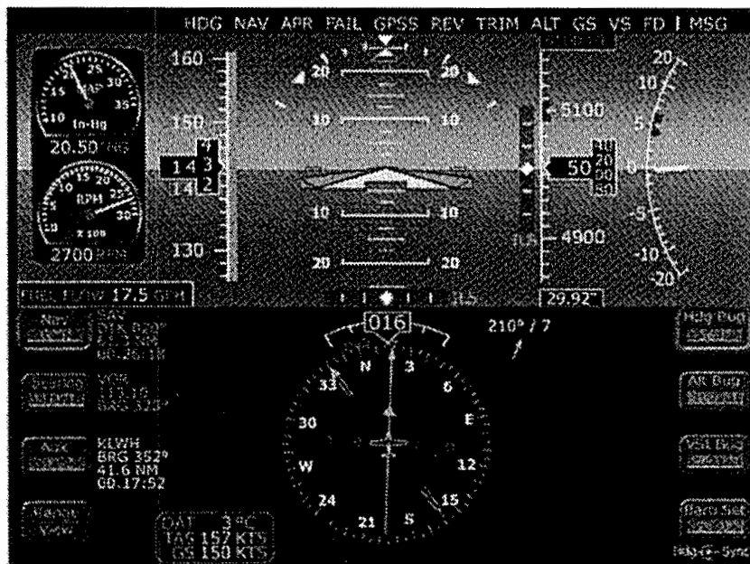
Figure 1 - Entegra 700-00006-0XX-( ) Primary Flight Display
