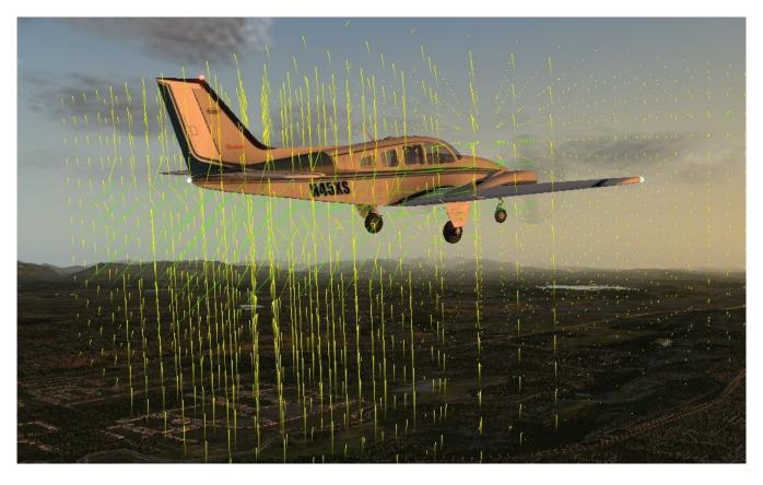
Figure 5.8: The flow field around a Baron 58
