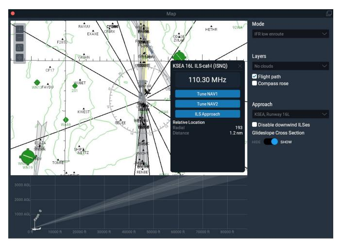
Figure 7.1: The map window in IFR low enroute mode, with the KSEA airport inspector window open
