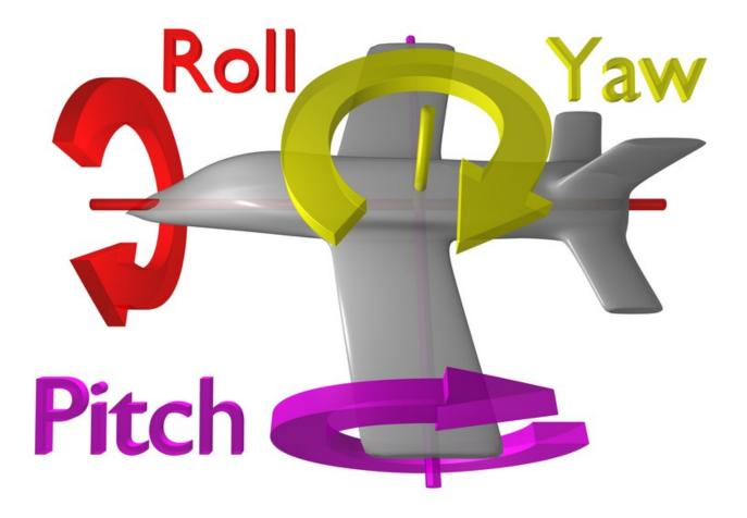
**Figure G.1**: This image illustrates the pitch, roll, and yaw axes of an airplane (which also apply to helicopters). Thanks to Wikipedia contributor <u>ZeroOne</u> for releasing this image under the Creative Commons Attribution 3.0 Unported license.
